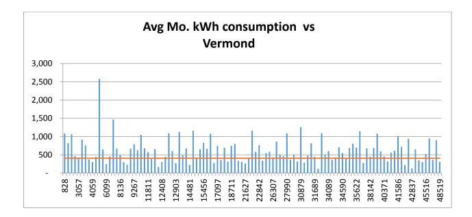
Avg. Monthly electric bill (2014 -2016) by Location/customer ID compared to the estimated average electric bill of a 980 sq ft "cottage style" Vermod, including heating, cooling, lighting and appliances (orange line).
